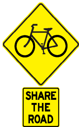
MUTCD Sign Types W11-1 and W16-1 (Share the Road with Bicyclists Assembly)
